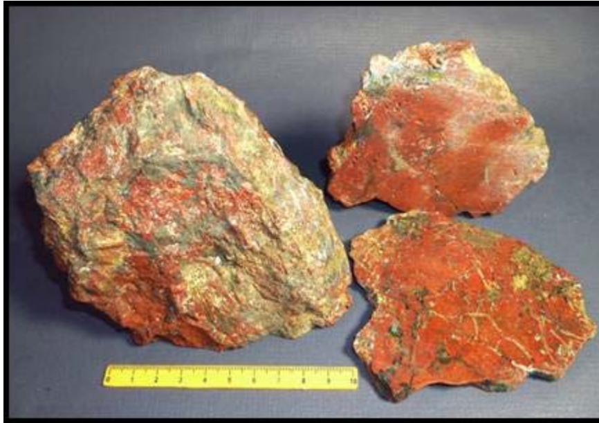
Figure 1 : Sample of the bad jasper. Please note the white chalcedony veins on the surface of the cut jasper ( below right )
