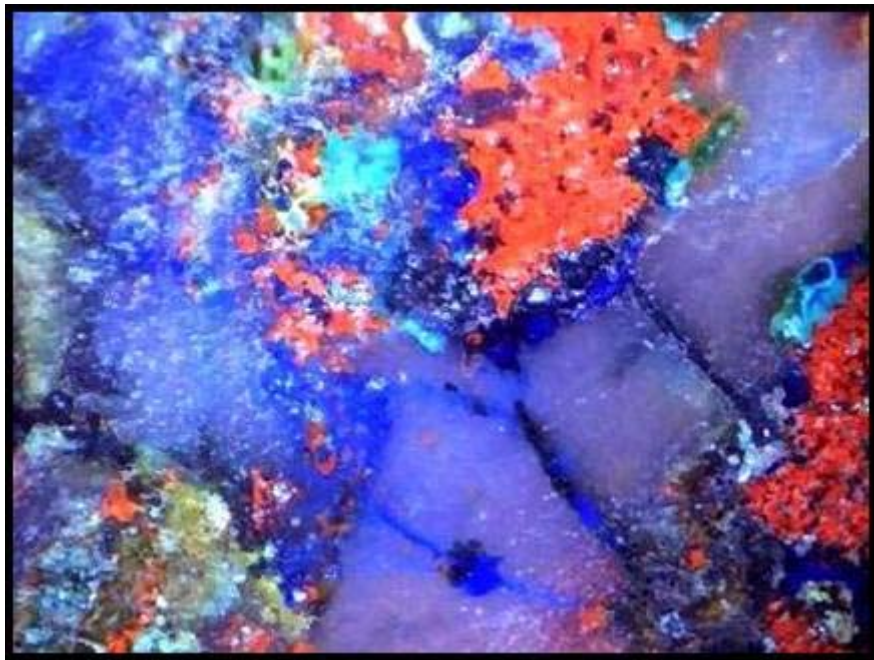
Figure 3 : Relatively thick chalcedony vein with cracks that were filled by Azurite . Please note the greenish blue Malachite.
